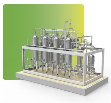
The hydrogen generated by water electrolysis contains an oxygen impurity, typically below 0.2%, and a small amount of saturated water. Oxygen and hydrogen react rapidly to produce water through a catalytic reaction in a de-aerator. Molecular sieves in the dryer are used to adsorb the residual water contained in the hydrogen. After purification, hydrogen achieves a 5.0 grade purity level.
