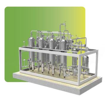
The hydrogen generated by water electrolysis contains an oxygen impurity, typically below 0.2%, and a small amount of saturated water. Oxygen and hydrogen react rapidly to produce water through a catalytic reaction in a de-aerator. Molecular sieves in the dryer are used to adsorb the residual water contained in the hydrogen. After purification, hydrogen achieves a 5.0 grade purity
