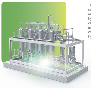
The hydrogen generated by water electrolysis contains an oxygen impurity, typically below 0.2%, and a small amount of saturated water. Oxygen and hydrogen react rapidly to produce water through a catalytic reaction in a de-aerator. Molecular sieves in the dryer are used to adsorb the residual water contained in the hydrogen. After purification, hydrogen achieves a purity level of 99.999%.
